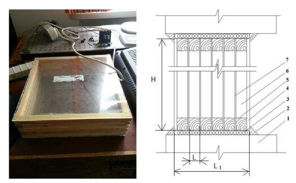
Fig. 1. Experimental multiglass window: 1 – window column; 2 – timber sealing strip; 3 – package sealing; 4 – thick outer glass (4 mm); 5 – timber spacer; 6 – air gap; 7 – thin inner glass (2 mm); *H* – height (300 mm); *L<sub>t</sub>* – total width of window (96 mm); *L* – width of each air gap between glasses (16 mm)
