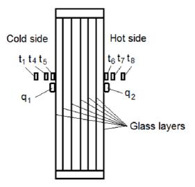
Fig.2. **Position of sensors:** t1, t8 – sensors of air temperatures; t4, t7 – sensors of air temperatures near outer glass (distance between glass surface and sensor approx.2 mm); t5, t6 – sensors of temperatures on glass outer surfaces; q1, q2 – heat flow meters
